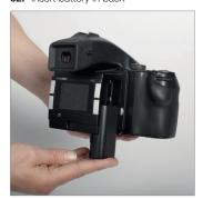
03. Insert batteries in camera
